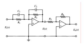
$$\begin{split} \frac{E_0(s)}{E_i(s)} &= \frac{R_2R_4}{R_1R_3} \, \frac{R_1C_1 + 1}{R_2C_2 + 1} = \frac{R_4C_1}{R_3C_2} \, \frac{s + \frac{1}{R_1C_1}}{s + \frac{1}{R_2C_2}} = K_c\alpha \, \frac{Ts + 1}{\alpha Ts + 1} = K_c \, \frac{s + \frac{1}{T}}{s + \frac{1}{\alpha T}} \\ T &= R_1C_1, \qquad \alpha T = R_2C_2, \qquad \alpha = \frac{R_2C_2}{R_1C_1} < 1 \\ K_c\alpha &= \frac{R_2R_4}{R_1R_3}, \qquad K_c &= \frac{R_4C_1}{R_3C_2} \end{split}$$
